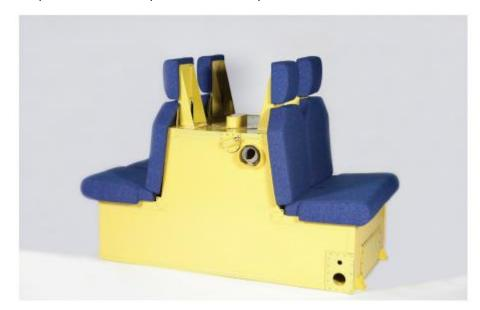
The seat tank allows the Super Puma to carry 545 liters (144 U.S. gallons / 120 Imperial gallons) of additional fuel on board which can be transferred to the main tanks.
